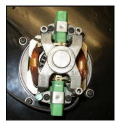
1. Remove the motor cover from the vacuum lid to see the armature, pictured above. Each of the two interrupter brushes is held in place with a metal strap secured by two screws. The brushes' plastic case is green in this picture, but the casing can come in other colors, such as brown, black or white.
