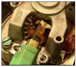
**4.** When the connector is completely removed from the brush casing, the strap can be unscrewed and removed, so a new brush can be installed.
