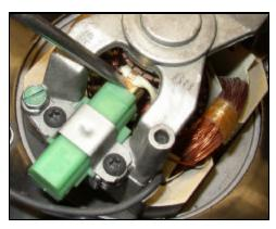
**3.** To replace a worn brush, first loosen the brass connector that is connected to the motor. A screwdriver is a good tool for pushing the connector away from the brush and toward the center.
