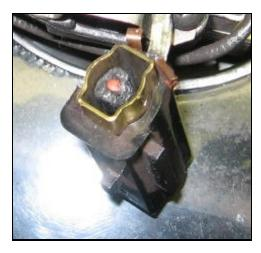
2. When the interrupter brush is worn, a plastic core is exposed inside the carbon brush. This core stops ("interrupts") the motor before the metal collar on the brush damages the armature. Worn brushes must be replaced (part #737-0051) before the motor will run again.
